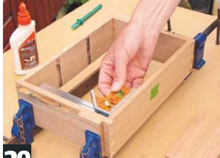
20 Clean up inner surfaces and check for fit. Glue and cramp up tray, checking for square
